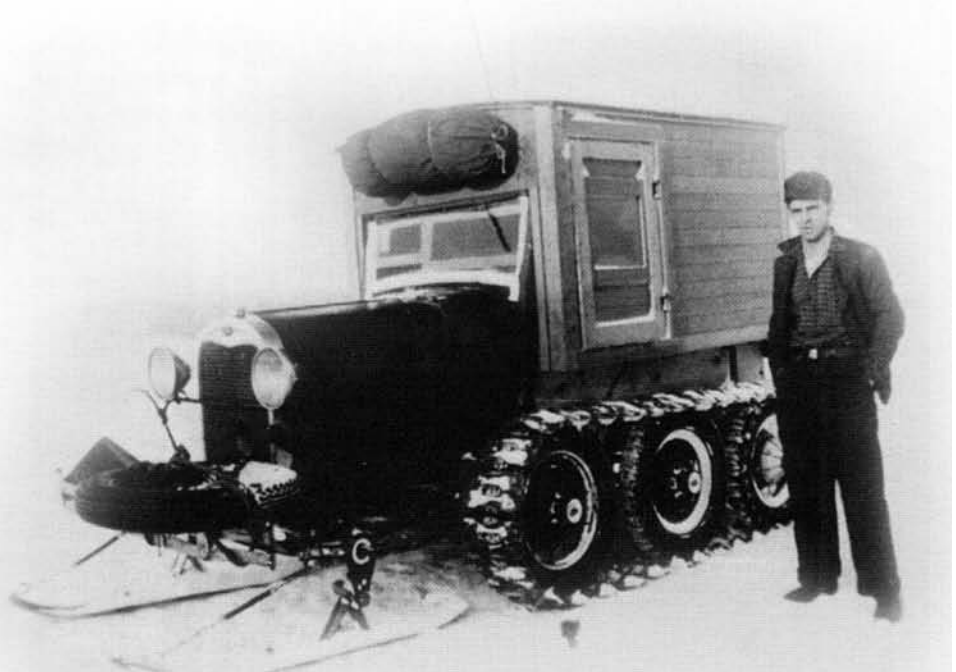
Dr. Hamman's snow machine assembled on a Model A chassis (circa 1935) and his driver Alex Campbell. Note the Arctic bedroll mounted over the windscreen.
